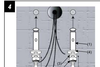
Drive the expansion anchors (1) into the holes. (Note: do not detach hex nut (2), spring washer (3) and metal washer (4) for this step).
