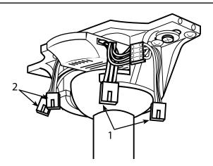
While fan is hanging on bracket, plug 4-pole connector from the mounting bracket into the 4-pole plug connector from the remote receiver (1). Plug the 4-pole plug connector from the remote receiver into the 4-pole plug connector from the fan (2).
