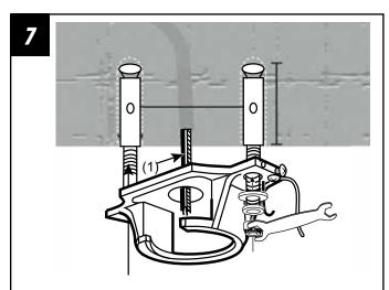
Pull the supply mains (1) through the center of the ceiling, and align the two oval holes in the mounting bracket with the expansion anchors, re-install metal washer, spring washer and hex nut, tighten the hex nut until the mounting bracket is fix stably.
