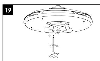
Attach the light kit onto the light kit pan by placing the key slot holes from the light kit onto the two protruding screw heads from the light kit pan. Twist the light kit close-wise until the screw heads engage the key slots. Install the screw removed from the light kit pan (step#18) into the closed hole in the light kit. Tighten all screws to complete attachment of the light kit.
