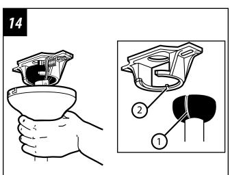
Carefully lift fan assembly onto mounting bracket. Rotate fan until notch on downrod ball (1) engages the ridge (2) on the mounting bracket. This will allow for hands free wiring.
