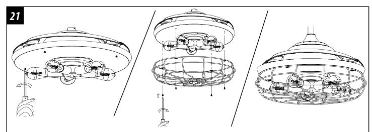
Remove the 4 fixing screws from the light kit pan. Keep them for next step.
