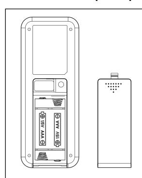
Restore electrical power to the outlet box by turning on the electricity at the main fuse box. To make the fan operational, open battery door by pressing and sliding down the battery door. Install two AAA 1.5V batteries (not included) into the hand-held remote transmitter(if not used for long periods of time, remove the batteries to prevent damage to the transmitter).
