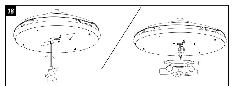
Remove ONLY the one screw on the light kit pan identified with paper tag, and loosen (do not remove) the other two. Find the Molex connector from the motor and the Molex connector from the light kit. Slide them together.
