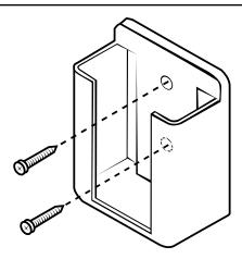
Note: Install two AAA batteries by removing battery cover on back of transmitter, installing batteries, and replacing battery cover. If desired, install the transmitter holder onto the wall with included screws.
