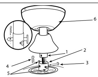
Loose (but do not remove) the set screws (5) from the down rod coupling. Insert downrod (1) into downrod coupling (2). Make sure to align hole in downrod with the hole in downrod coupling. Install cross pin (3) through coupling and downrod. Insert clamp pin (4) into cross pin until it snaps into place. Tighten set screws (5) in coupling. Slide coupling cover (6) over the downrod coupling.
