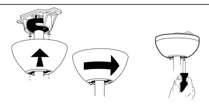
Loosen the 2 screws on the bottom of mounting bracket but do not remove them. Raise the canopy up and align the keyholes on the bottom of the canopy with the 2 screws on the bottom of mounting bracket. Rotate the canopy until both screws from the mounting bracket drop into the slot recesses. Tighten screws securely.
