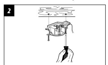
Drill two mounting holes in the ceiling joist and securely screw the mounting bracket to the ceiling using the washers and wood screws provided. The mounting plate should be able to hold a weight of at least 15.9kgs (35 lbs). NOTE - Proper care must be taken when mounting to concrete ceilings. For safe mounting, these ceilings may require stronger screws and plastic plugs or anchors than supplied with the product.
