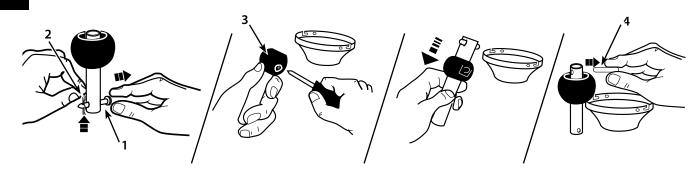
Remove clamp pin (2) and cross pin (1) from downrod. Loosen set screws in downrod ball (3) until ball moves easily up and down the downrod. Slide downrod ball down, exposing cross pin (4). Do not remove ball completely. Remove cross pin and save for later use.
